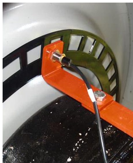
Inductive sensor with LED detecting metal
