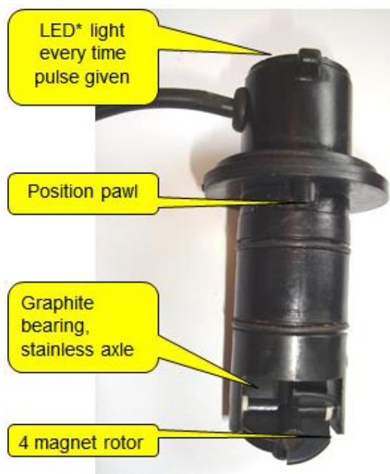
Flow sensor with rotor at bottom
