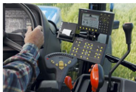
Primary and secondary functions with Grip and SetBox
