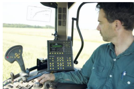
Primary and secondary functions with Grip and SetBox
