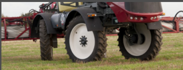
4-wheel steering – field mode
